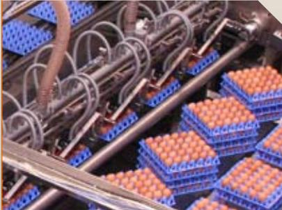
Accumulator combining high filling ratio with gentle egg handling
