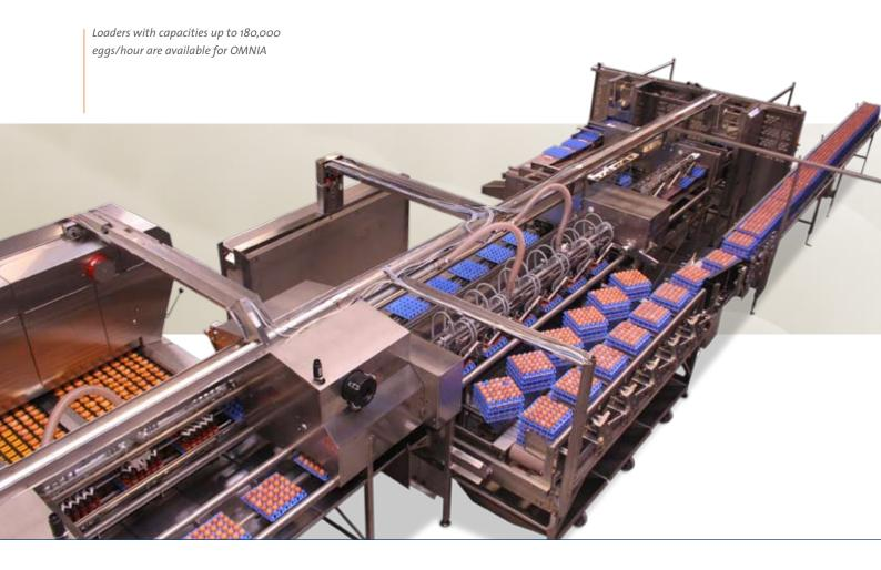
In the machine itself a heavy duty industrial network handles the signals to control the machine. Because such a network prevents enormous bundles of cables and also offers an integral self-check and diagnostic system, a secure and reliable operation of the machine is ensured.
